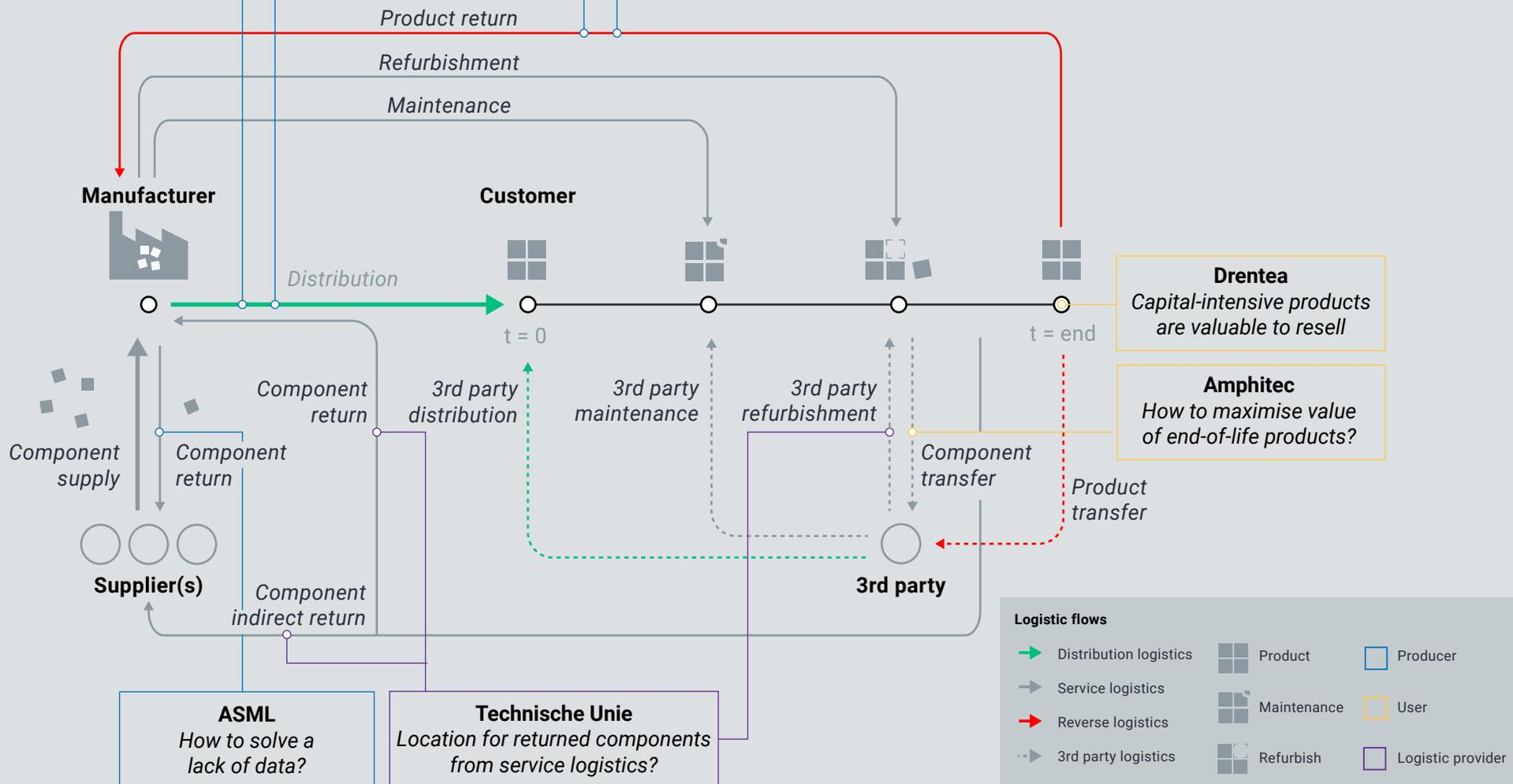
Figure 6 | Logistical challenges in a circular capital-intensive manufacturing industry.
