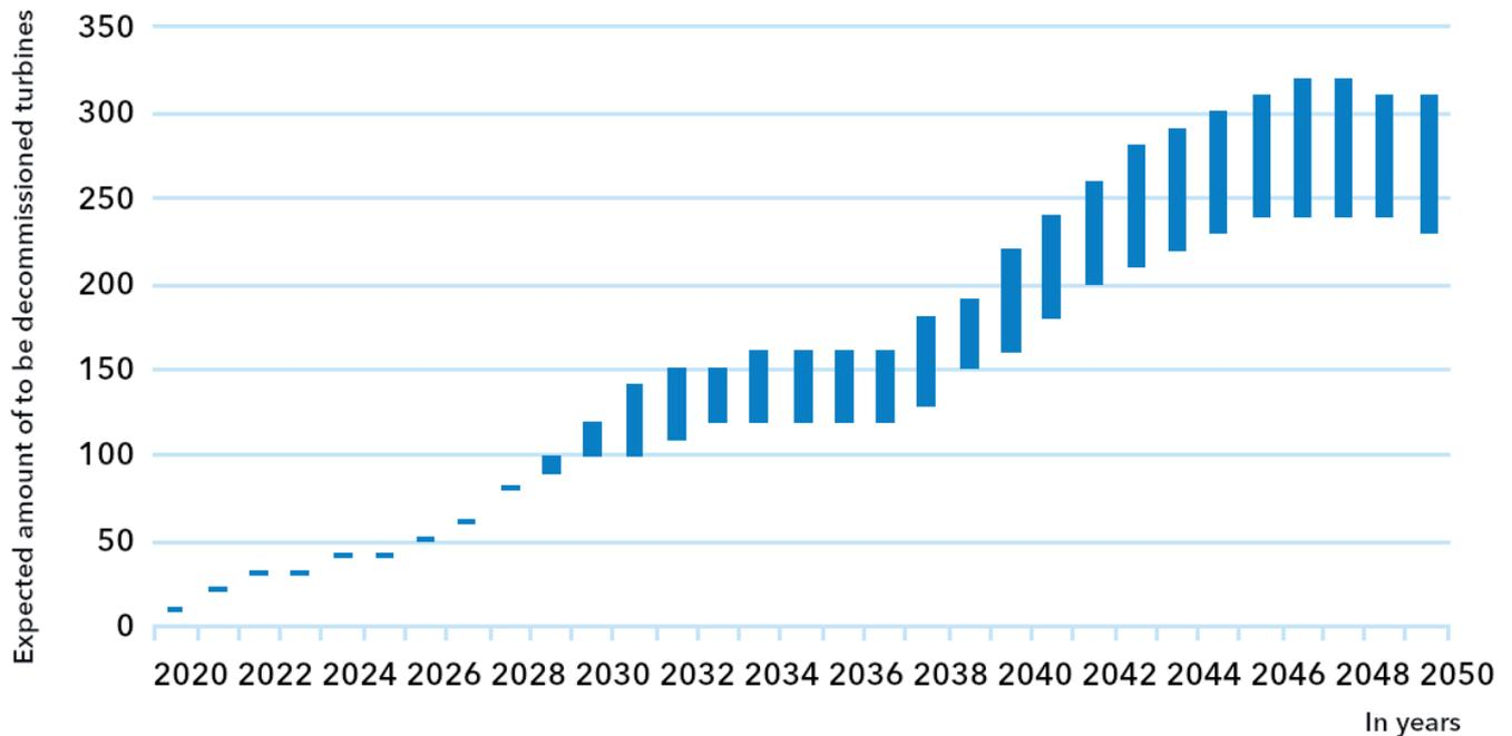
Figure 2: The residual flow of the expected amount of offshore wind turbines in the southern North Sea area (Hajonides et al., 2020)<sup>6</sup>
