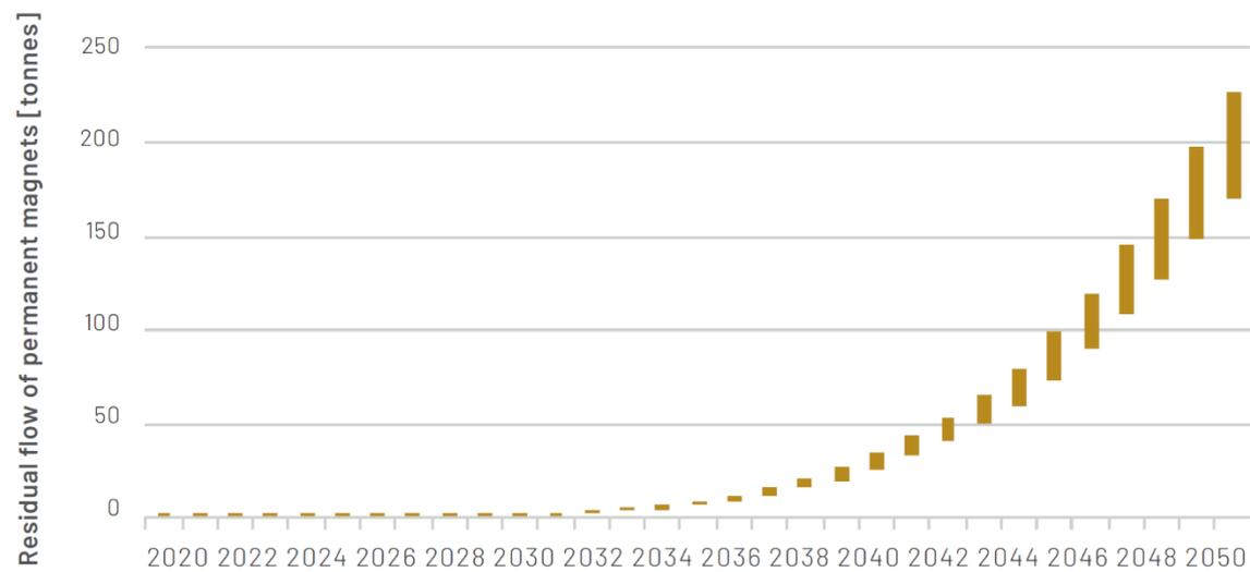
Figure 24: Residual flow of neodymium alloy permanent magnets [tonnes] (NdFeB) resulting from offshore wind farms decommissioning in the Southern North Sea (Hajonides et al., 2020).
